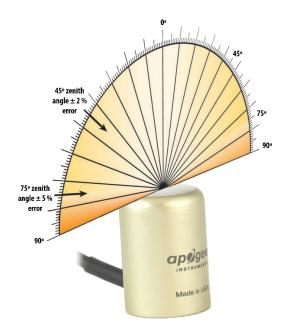
Directional, or cosine, response is defined as the measurement error at a specific angle of radiation incidence. Error for Apogee SQ series quantum sensors is approximately  $\pm 2$ % and  $\pm 5$ % at solar zenith angles of 45° and 75°, respectively.
