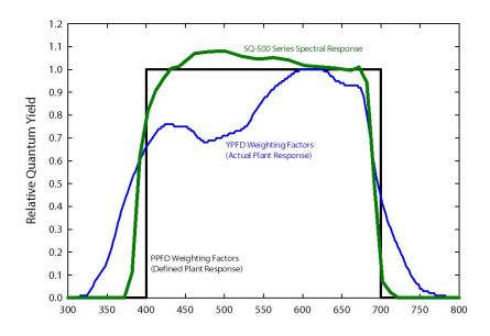
Radiation weighting factors for PPFD (black line, defined plant response to radiation), YPFD (blue line, measured plant response to radiation), and Apogee SQ-500 Series Quantum Sensors (green line, sensor sensitivity to different wavelengths of radiation).
