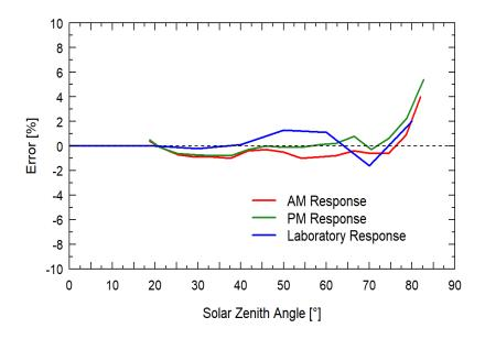
Mean cosine response of seven apogee SQ-500 quantum sensors. Cosine response measurements were made on the rooftop of the Apogee building in Logan, UT. Cosine response was calculated as the relative difference of SQ-500 quantum sensors from the mean of replicate reference quantum sensors (LI-COR models LI-190 and LI-190R, Kipp & Zonen model PQS 1).
